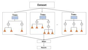
**Fig. 3** Schematic diagram of random forests (RFs). An RF is an ensemble learning approach that consists of multiple decision trees. In the process of training the RF model, each decision tree is trained in sequence, and the training samples of each tree are extracted from the original datasets by a randomized sampling method. The features used in each decision tree are also obtained by random sampling. The joint prediction of multiple decision trees improves the accuracy of the RF model
