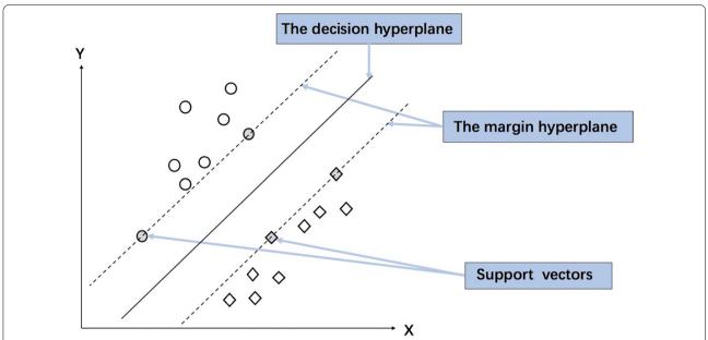
**Fig. 2** Schematic diagram of a support vector machine (SVM). Although a decision hyperplane with maximal margin separates every sample into two classes, the support vector is the sample point on the margin hyperplane, which is the largest margin of classification under the constraints. The final SVM model is only related to support vectors
