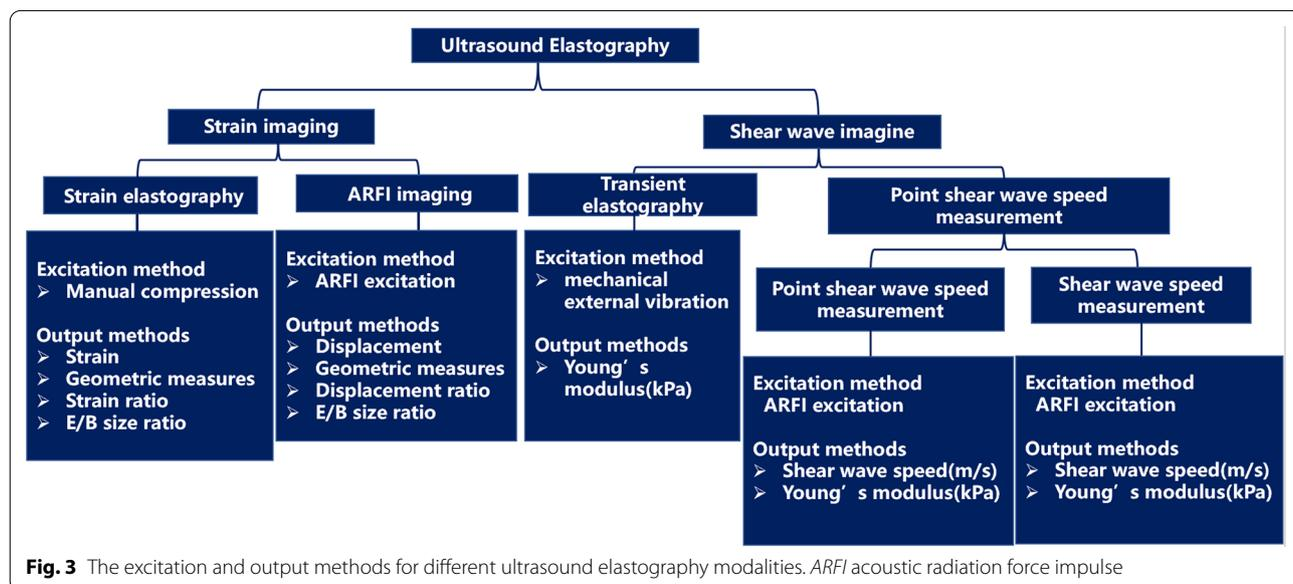
**Fig. 3** The excitation and output methods for different ultrasound elastography modalities. *ARFI* acoustic radiation force impulse
