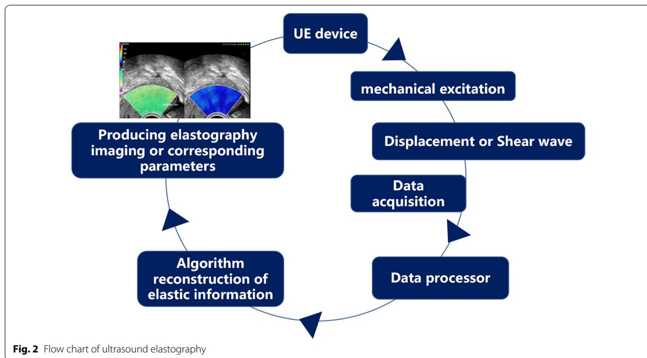
**Fig. 2** Flow chart of ultrasound elastography
