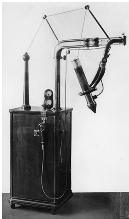
Fig. 10 Dental X-ray system from Ritter Dental with a Philips Metalix A tube. The cathode was grounded, but the radiator at the end of the tube had anode potential (system from around 1921–1924) [48]
