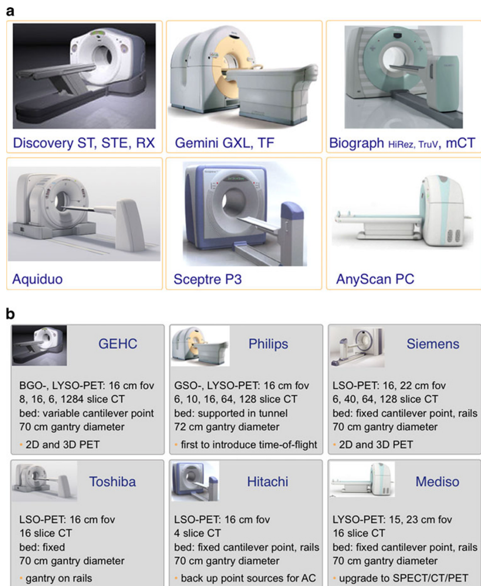
Fig. 1 a Selected PET/CT designs offered by GE Healthcare, Philips Healthcare Systems, Siemens Healthcare Solutions, Toshiba, Hitachi and Mediso. b Selected system design parameters for the PET/CT systems in a
